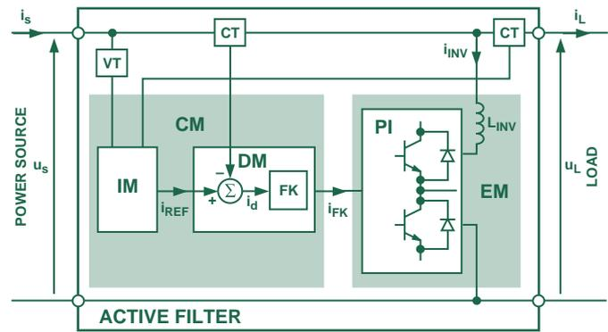
Figure 1. Block diagram of the active filter.
